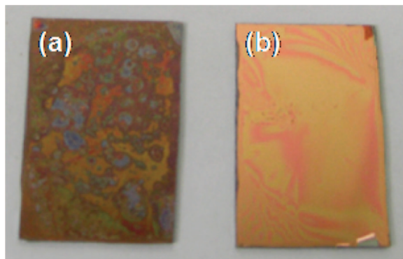
Figure 14. Photograph of their corrosion-tested samples: (a) PHA polymer film with 10 wt % PTMA as PAG on the 0.3 \mu\text{m} Cu-coated silicon wafer; (b) PHA polymer film with 10 wt % DNCDP as PBG on the 0.3 \mu\text{m} Cu-coated silicon wafer.
